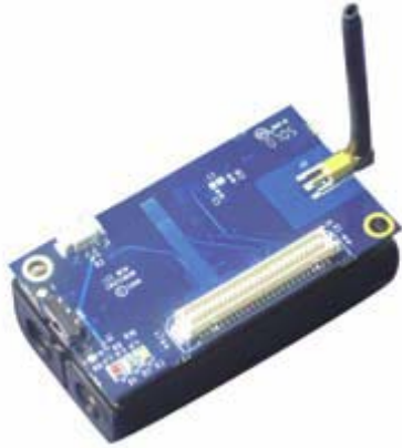
Figure 2. The IRIS 2.4 GHz Mote module used in the Street Corners implementation.
